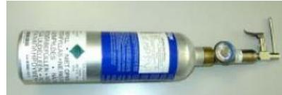
This information applies to the Dräger test gas bottles with 34 l of ethanol test gas (part number 68 10 920) and with 103 l of ethanol test gas (part number 68 10 695). It describes how to prepare the test gas bottles in a safe way for recycling or disposal by "destroying" the internal bottle valve and render it useless.
