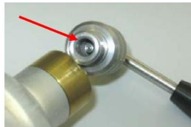
Retract the centre punch of the recycling tool completely into the body by turning the knurled body until it stops.
