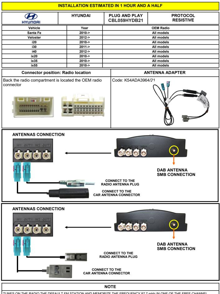
TUNES ON THE RADIO THE DEFAULT FM STATION AND MEMORIZE THE FREQUENCY 87.7 mHz IN ONE OF THE FREE CHANNEL (EXAMPLE POSITION 1).
