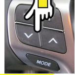
**PRESS QUICKLY THE BUTTON OF MEDIADAB TO JUMP MUTE FUNCTION, LED BECOMES ORANGE AND TURNS IMMEDIATELY RED**
