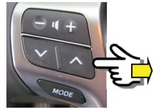
**PRESS MODE THE LED BECOMES ORANGE: PLEASE KEEP IT PRESS FOR 1 SECOND AND RELEASE IT WHEN THE LED IS RED**
